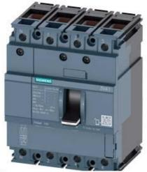
CIRCUIT BREAKER 3VA1 IEC FRAME 100 BREAKING CAPACITY CLASS S ICU=36KA @ 415 V 4-POLE, LINE PROTECTION TM210, FTFM, IN=16A OVERLOAD PROTECTION IR=16A FIXED SHORT CIRCUIT PROTECTION II=10 X IN NEUTRAL UNPROTECTED CABLE CONNECTION
