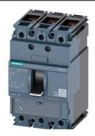
CIRCUIT BREAKER 3VA1 IEC FRAME 160 BREAKING CAPACITY CLASS S ICU=36KA @ 415 V 3-POLE, LINE PROTECTION TM220, ATFM, IN=32A OVERLOAD PROTECTION IR=22,4A ...32A SHORT CIRCUIT PROTECTION II=10 X IN BUSBAR CONNECTION
