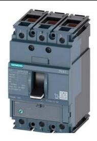
CIRCUIT BREAKER 3VA1 IEC FRAME 160 BREAKING CAPACITY CLASS M ICU=55KA @ 415 V 3-POLE, LINE PROTECTION TM220, ATFM, IN=63A OVERLOAD PROTECTION IR=44,1A ...63A SHORT CIRCUIT PROTECTION II=10 X IN CABLE CONNECTION
