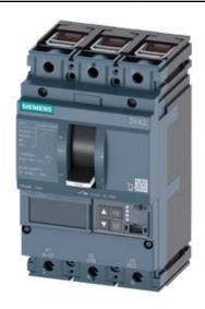
CIRCUIT BREAKER 3VA2 IEC FRAME 160 BREAKING CAPACITY CLASS H ICU=85KA @ 415 V 3POLE, LINE PROTECTION ETU560, LSIG, IN=25A OVERLOAD PROTECTION IR=10A ...25A SHORT CIRCUIT PROTECTION ISD=0,6..10X IN, II=1,5...12X IN NEUTRAL PROTECTION OPTIONAL WITH EXT. CT,UPTO 160% GROUNDFAULT, SWITCHABLE IG=0,2... 1 X IN, TG=0,050,8MS CABLE CONNECTION
