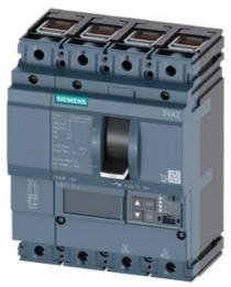
CIRCUIT BREAKER 3VA2 IEC FRAME 160 BREAKING CAPACITY CLASS C ICU=110KA @ 415 V 4POLE, LINE PROTECTION ETU850, LSI, IN=25A OVERLOAD PROTECTION IR=10A ...25A SHORT CIRCUIT PROTECTION ISD=0,6..10X IN, II=1,5..12X IN NEUTRAL PROTECTION ADJUSTABLE (OFF, UPTO 160%) CABLE CONNECTION
