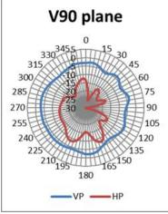
VP: Vertical Polarization HP: Horisontal Polarization
