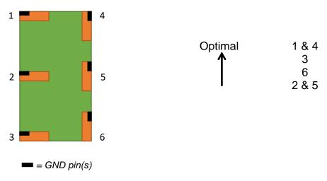
The antenna should be aligned with the PCB edge if possible, preferably with the GND pin(s) close to a corner.
