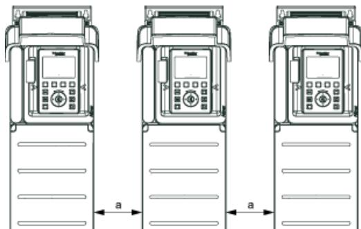
Mounting Type B: Side by Side IP20
