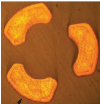
Au/Ni Barrier (Uniform plating thickness)
