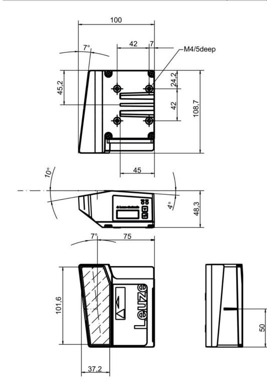
Part no.: 50139945 – BPS 338i SM 100 H – Bar code positioning system
