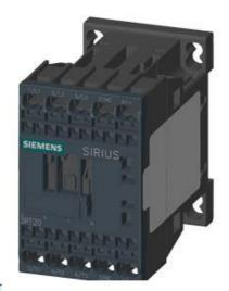
COUPLING RELAY, AC-3, 4KW/400V, 1NC, DC 12V, 0.7...1.25\*US, W. INTEGR. SUPPRESSORDIODE, SZ S00, SPRING-LOADED TERMINAL
