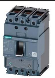
CIRCUIT BREAKER 3VA1 IEC FRAME 160 BREAKING CAPACITY CLASS S ICU=36KA @ 415 V 3-POLE, LINE PROTECTION TM240, ATAM, IN=25A OVERLOAD PROTECTION IR=17,5A ...25A SHORT CIRCUIT PROTECTION II=6,4...12,8 X IN CABLE CONNECTION
