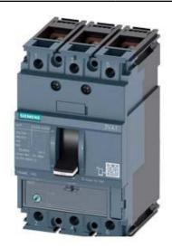
CIRCUIT BREAKER 3VA1 IEC FRAME 160 BREAKING CAPACITY CLASS M ICU=55KA @ 415 V 3-POLE, LINE PROTECTION TM220, ATFM, IN=25A OVERLOAD PROTECTION IR=17,5A ...25A SHORT CIRCUIT PROTECTION II=10 X IN BUSBAR CONNECTION
