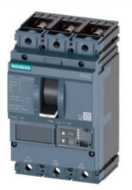
CIRCUIT BREAKER 3VA2 IEC FRAME 160 BREAKING CAPACITY CLASS C ICU=110KA @ 415 V 3POLE, LINE PROTECTION ETU860, LSIG, IN=40A OVERLOAD PROTECTION IR=16A ...40A SHORT CIRCUIT PROTECTION ISD=0,6..10X IN, II=1,5..12X IN NEUTRAL PROTECTION OPTIONAL WITH EXT. CT,UPTO 160% GROUNDFAULT, SWITCHABLE IG=0,2... 1 X IN, TG=0,050,8MS BUSBAR CONNECTION
