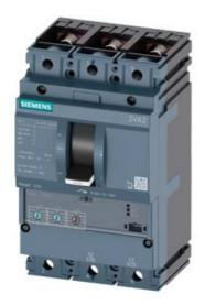
CIRCUIT BREAKER 3VA2 IEC FRAME 250 BREAKING CAPACITY CLASS M ICU=55KA @ 415 V 3POLE, LINE PROTECTION ETU320, LI, IN=160A OVERLOAD PROTECTION IR=64A ...160A SHORT CIRCUIT PROTECTION II=12 X IN BUSBAR CONNECTION
