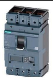
CIRCUIT BREAKER 3VA2 IEC FRAME 400 BREAKING CAPACITY CLASS C ICU=110KA @ 415 V 3-POLE, LINE PROTECTION ETU850, LSI, IN=400A OVERLOAD PROTECTION IR=160A ...400A SHORT CIRCUIT PROTECTION ISD=0,6..10X IN, II=1,5..10X IN NEUTRAL PROTECTION OPTIONAL WITH EXT. CT;UPTO 160% BUSBAR CONNECTION
