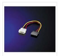
Adapter cable for converting the 4-pin HDD interface to the SATA power connector; 4-pin cable, connections: 4-pin HDD plug to 15-pin SATA power connector; length: 0.15 m
