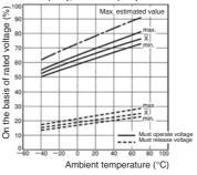
Ambient Temperature vs. Must Set or Must Reset Voltage G6KU-2G (F/P)-Y
