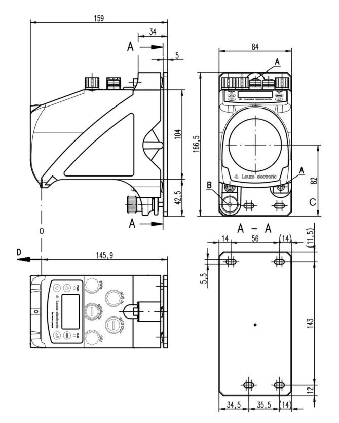
A M 5 screw for alignment
