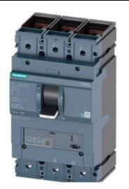
CIRCUIT BREAKER 3VA2 IEC FRAME 400 BREAKING CAPACITY CLASS M ICU=55KA @ 415 V 3-POLE, LINE PROTECTION ETU320, LI, IN=250A OVERLOAD PROTECTION IR=100A ...250A SHORT CIRCUIT PROTECTION II=12 X IN BUSBAR CONNECTION
