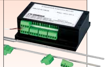
OM-CP-OCTRTD 8-channel data logger, visit omega.com/om-cp-octrtd
