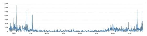
We can see the concentration of dust is very low in the evening, but it's higher in the afternoon. Maybe you can set a threshold value while the concentration is beyond a value. Also, if you wanna set the sensor more sensitive you can add a fan on the sensor, and add a 10k resistor between the Pin5 and Ground. More information please visit the blog of A.J.
