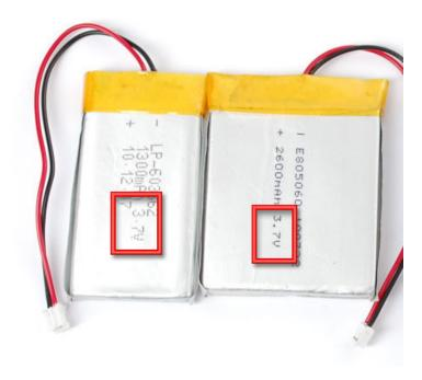
For example, here is a profile of the voltage for a 'classic' **3.7V/4.2V** battery. The voltage starts at 4.2 maximum and quickly drops down to about 3.7V for the majority of the battery life. Once you hit 3.4V the battery is dead and at 3.0V the cutoff circuitry disconnects the battery (more on that later.
