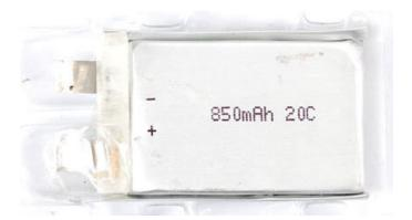
Important Note! Unless you are specifically building an RC device like a quadcopter, we suggest that you should never use RC lithium ion batteries for DIY projects. They do not have protection circuitry and are designed to not be safe. They have a much higher risk of exploding or catching on fire. If you need more current capability, just go with a larger lithium ion/polymer battery
