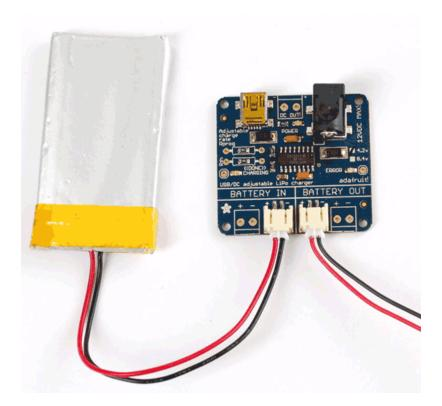
If you want to use the battery while also having it connected to the charger (less plugging and unplugging that way) you can simply use the **BATTERY OUT** connecion on the right. The **IN** and **OUT** ports are connected together on the circuit board so it acts as a *pass-through*
