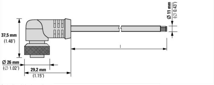
Supply cable, prefabricated on one side
