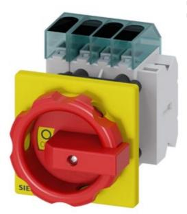
Switch disconnector 3LD3, main switch 3-polig + N, lu 63A operational switch at AC-23 A at 400 V 22,0 kW front mounted Base mounting with center-hole 22,5 mm knob-operated mechanism red/yellow 66 x66 mm with auxiliary 1NO+1NC
