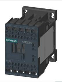
COUPLING RELAY, AC-3, 4KW/400V, 1NC, DC 24V, 0.7...1.25\*US, W. INTEGR. SUPPRESSORDIODE, SZ S00, SPRING-LOADED TERMINAL
