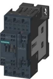
CONT. F. RAILW. A., AC-3, 7.5KW/400V, 1NO+1NC, . DC 110V, 0,7...1,25\*US, M. VARISTOR INTEGRATED, 3-POLE SIZE S0, SPRING-TYPE TERM.
