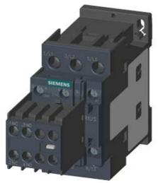
CONTACTOR, AC-3, 15KW/400V, 2NO+2NC, AC 110V 50HZ, 3-POLE, SZ S0 SCREW TERMINAL REMOVABLE AUX. SWITCH
