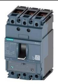
CIRCUIT BREAKER 3VA1 IEC FRAME 160 BREAKING CAPACITY CLASS S ICU=36KA @ 415 V 3-POLE, LINE PROTECTION TM240, ATAM, IN=80A OVERLOAD PROTECTION IR=56A ...80A SHORT CIRCUIT PROTECTION II=5...10 X IN BUSBAR CONNECTION
