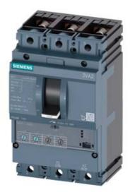
CIRCUIT BREAKER 3VA2 IEC FRAME 100 BREAKING CAPACITY CLASS H ICU=85KA @ 415 V 3POLE, LINE PROTECTION ETU330, LIG, IN=25A OVERLOAD PROTECTION IR=10A ...25A SHORT CIRCUIT PROTECTION II=1,5...12 X IN GROUNDFAULTPROTECTION IG=0,2... 1 X IN, TG=0,1/0,3MS BUSBAR CONNECTION
