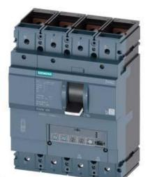
CIRCUIT BREAKER 3VA2 IEC FRAME 400 BREAKING CAPACITY CLASS C ICU=110KA @ 415 V 4-POLE, LINE PROTECTION ETU350, LSI, IN=250A OVERLOAD PROTECTION IR=100A ...250A SHORT CIRCUIT PROTECTION ISD=1,5... 10 X IR, II=12 X IN NEUTRAL PROTECTION ADJUSTABLE(OFF,50%,100%) BUSBAR CONNECTION
