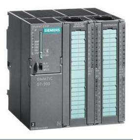
SIMATIC S7-300, CPU 314C-2 PTP COMPACT CPU WITH MPI, 24 DI/16 DO, 4AI, 2AO, 1 PT100, 4 FAST COUNTERS (60 KHZ), INTEGRATED INTERFACE RS485, INTEGRATED 24V DC POWER SUPPLY, 192 KBYTE WORKING MEMORY, FRONT CONNECTOR (2 X 40PIN) AND MICRO MEMORY CARD REQUIRED
