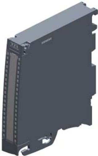
SIMATIC S7-1500, ANALOG INPUT MODULE AI 4 X U/I/RTD/TC, 16 BITS OF RESOLUTION, ACCURACY 0.3 %; 4 CHANNELS IN GROUPS OF 4; 2 CHANNELS FOR RTD MEASURING, COMMON MODE VOLTAGE APPR. 10 V; DIAGNOSIS, PROCESSALARMS INCL. FRONT CONNECTOR PUSH-IN, FEEDING ELEMENT, SHIELDING ELEMENT, SHIELDING CLAMP
