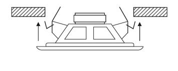
Push the speaker into the hole allowing the spring clips to grip the ceiling tile/wall panel. The speaker should be checked to ensure it is secure and cannot be dislodged or fall.
