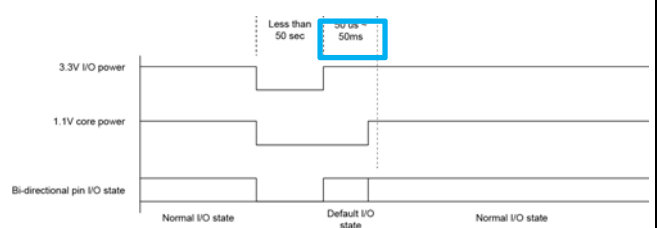
Figure Error! No text of specified style in document.-12 Recommended Power Sequence
