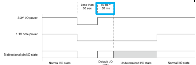
Figure Error! No text of specified style in document.-11 Timing Sequence with Undetermined I/O State
