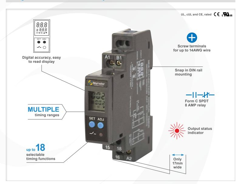
Trumeter's new range of digital time relays offer 8 or 18 operating modes, easily configured on the 3 digit LCD display: a wide range of 0.1s - 999Hr to suit all applications; a clear indication of the relay status via the front panel LED; can accept a wide range of operating voltages for most installations. The keylock feature means settings cannot be tampered with, for 100% reliable operation.
