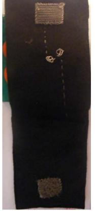
Conductive Hoop & Loop (Velcro™) can be used as a switch, it works in exactly the same way as the press stud. As explained earlier in Diagram 3.
