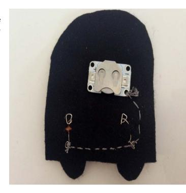
Sew a couple of stitches beyond the last LED leg and then knot tightly. Cut thread.
