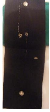
A metal sew on press stud can be used as a switch as explained earlier in Diagram 3.
