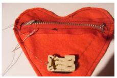
9. (The final steps) Thread a sewing needle with the conductive thread, ensuring the eye is narrow enough to go through the metal terminal. Connect to the terminal with a couple of Knots, by just catching the top layer of the felt it secures the holder firmly into position.
