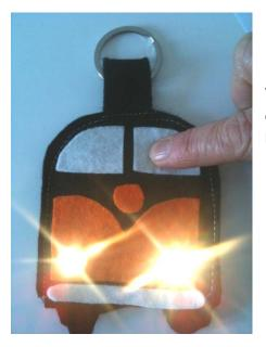
You will see that when the soft pad is pressed in the camper van window, it acts as a switch to turn the van lights on!
