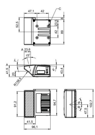
A Optical axis B Deflection angle of the laser beam:  $\pm$  30  $^\circ$
