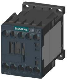
CONTACTOR, AC-3, 4KW/400V, 1NO, AC110V, 50/60 HZ, 3-POLE, SZ S00 SCREW TERMINAL
