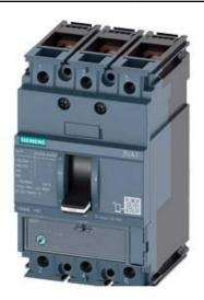
CIRCUIT BREAKER 3VA1 IEC FRAME 160 BREAKING CAPACITY CLASS S ICU=36KA @ 415 V 3-POLE, LINE PROTECTION TM220, ATFM, IN=160A OVERLOAD PROTECTION IR=112A ...160A SHORT CIRCUIT PROTECTION II=10 X IN BUSBAR CONNECTION
