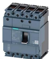
CIRCUIT BREAKER 3VA1 IEC FRAME 160 BREAKING CAPACITY CLASS H ICU=70KA @ 415 V 4-POLE, LINE PROTECTION TM210, FTFM, IN=63A OVERLOAD PROTECTION IR=63A FIXED SHORT CIRCUIT PROTECTION II=10 X IN NEUTRAL PROTECTION 100% CABLE CONNECTION
