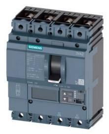
CIRCUIT BREAKER 3VA2 IEC FRAME 160 BREAKING CAPACITY CLASS L ICU=150KA @ 415 V 4POLE, LINE PROTECTION ETU850, LSI, IN=25A OVERLOAD PROTECTION IR=10A ...25A SHORT CIRCUIT PROTECTION ISD=0,6..10X IN, II=1,5..12X IN NEUTRAL PROTECTION ADJUSTABLE (OFF, UPTO 160%) BUSBAR CONNECTION
