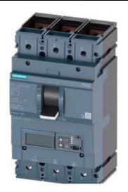
CIRCUIT BREAKER 3VA2 IEC FRAME 630 BREAKING CAPACITY CLASS H ICU=85KA @ 415 V 3-POLE, LINE PROTECTION ETU860, LSIG, IN=400A OVERLOAD PROTECTION IR=160A ...400A SHORT CIRCUIT PROTECTION ISD=0,6..10X IN, II=1,5..15X IN NEUTRAL PROTECTION OPTIONAL WITH EXT. CT;UPTO 160% GROUND-FAULT, SWITCHABLE IG=0,2... 1 X IN, TG=0,05-0,8MS BUSBAR CONNECTION
