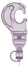
12 ton output force 1" stroke; 20,000 cycle Light Duty Compression Head 2 U-Die Compatible PN 1490745-1 IS 408-10111
