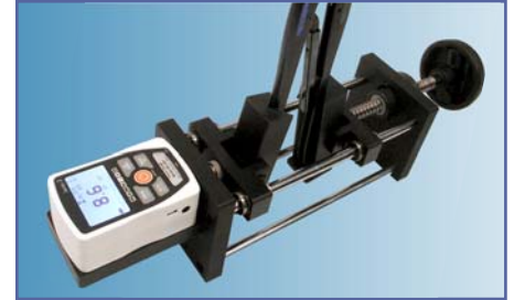
Handle force, measured at the factory, is a critical component of precise, reliable crimping.
