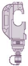
12 ton output force 1.5" stroke; 20,000 cycle Light Duty Compression Head U-Die Compatible PN 1490746-1 IS 408-10112
