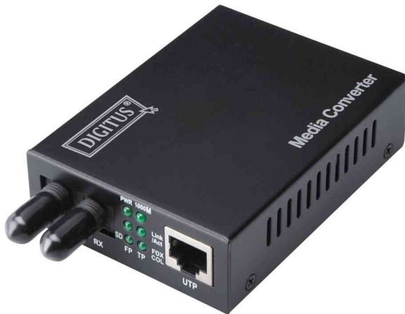
Fast Ethernet Medien Konverter, RJ45 - LWL-ST
