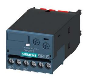
SOLID-STATE TIME-DELAY AUXILIARY SWITCH, ON-DELAY RELAY 1 CO CONTACT 24...240V AC/DC TIME RANGE 0.05...100 S FOR SNAPPING ONTO THE FRONT; FOR 3RT2 S00-S2 CONTACTORS SCREW TERMINALS INTEGRATED VARISTOR FOR DAMPING CONTACTOR COILS
