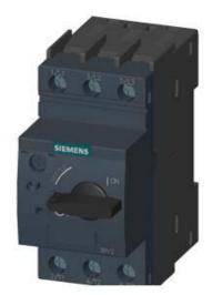
CIRCUIT-BREAKER SZ S0, FOR MOTOR PROTECTION, CLASS 10, A-REL. 0.9...1.25A, N-REL. 16A SCREW CONNECTION, STANDARD SW. CAPACITY
