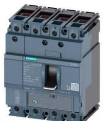
CIRCUIT BREAKER 3VA1 IEC FRAME 160 BREAKING CAPACITY CLASS M ICU=55KA @ 415 V 4-POLE, LINE PROTECTION TM220, ATFM, IN=160A OVERLOAD PROTECTION IR=112A ...160A SHORT CIRCUIT PROTECTION II=10 X IN NEUTRAL UNPROTECTED CABLE CONNECTION
