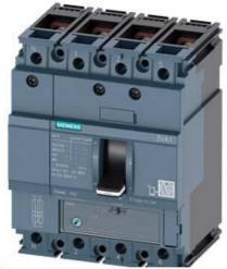
CIRCUIT BREAKER 3VA1 IEC FRAME 160 BREAKING CAPACITY CLASS S ICU=36KA @ 415 V 4-POLE, LINE PROTECTION TM220, ATFM, IN=20A OVERLOAD PROTECTION IR=14A ...20A SHORT CIRCUIT PROTECTION II=10 X IN NEUTRAL UNPROTECTED BUSBAR CONNECTION
