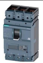
CIRCUIT BREAKER 3VA2 IEC FRAME 630 BREAKING CAPACITY CLASS C ICU=110KA @ 415 V 3-POLE, LINE PROTECTION ETU860, LSIG, IN=500A OVERLOAD PROTECTION IR=200A ...500A SHORT CIRCUIT PROTECTION ISD=0,6..10X IN, II=1,5..14X IN NEUTRAL PROTECTION OPTIONAL WITH EXT. CT;UPTO 160% GROUND-FAULT, SWITCHABLE IG=0,2... 1 X IN, TG=0,05-0,8MS BUSBAR CONNECTION
