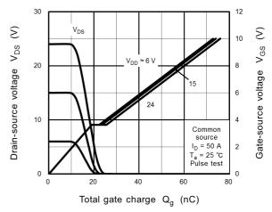
Fig. 8.10 Dynamic Input/Output Characteristics
