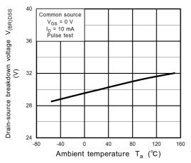
Fig. 8.7 V<sub>(BR)DSS</sub> - T<sub>a</sub>
