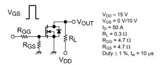
Fig. 6.2.1 Switching Time Test Circuit
