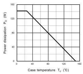
Fig. 8.15 P<sub>D</sub> - T<sub>c</sub> (Bottom drain) (Guaranteed Maximum)
