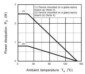
Fig. 8.14 P<sub>D</sub> - T<sub>a</sub> (Guaranteed Maximum)
