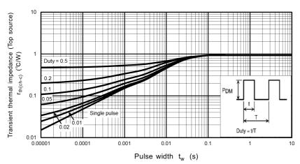
Fig. 8.13 r<sub>th</sub> - t<sub>w</sub> (Top source) (Guaranteed Maximum)
