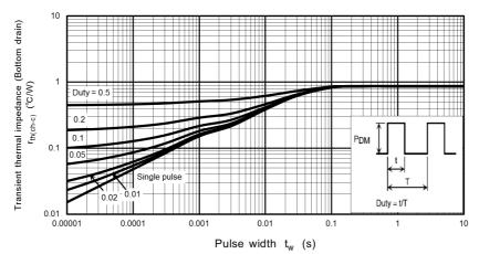
Fig. 8.12 r<sub>th</sub> - t<sub>w</sub> (Bottom drain) (Guaranteed Maximum)
